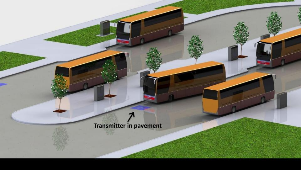
In this image, notice the blue tiles in front of the bus. As the bus pulls in the driver is guided to an aligned stopping position. The operator needs to take no action, charging commences immediately when the bus stops.
